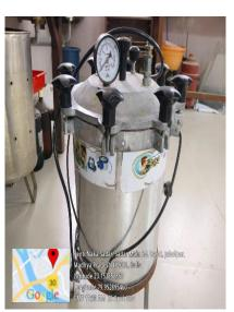
Autoclave for treating microbiological waste and sterilizing glassware
